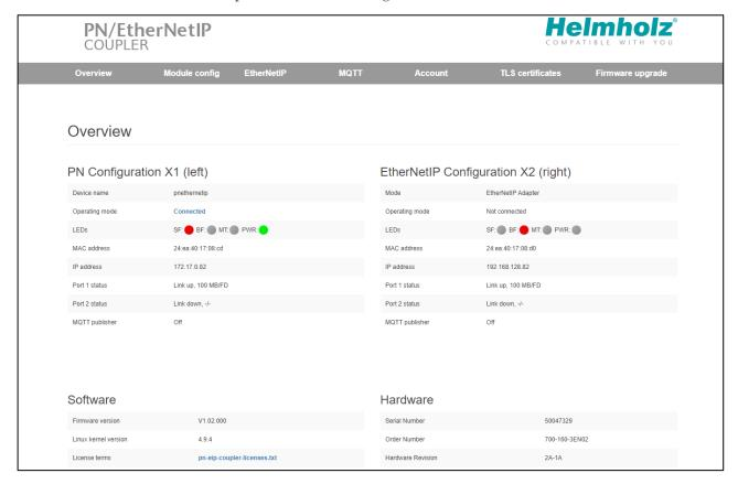
In the submenu "EtherNetIP" the network settings can be made, if they are not predefined by the PROFINET configuration, and the EDS file with the currently valid I/O configuration can be downloaded.
