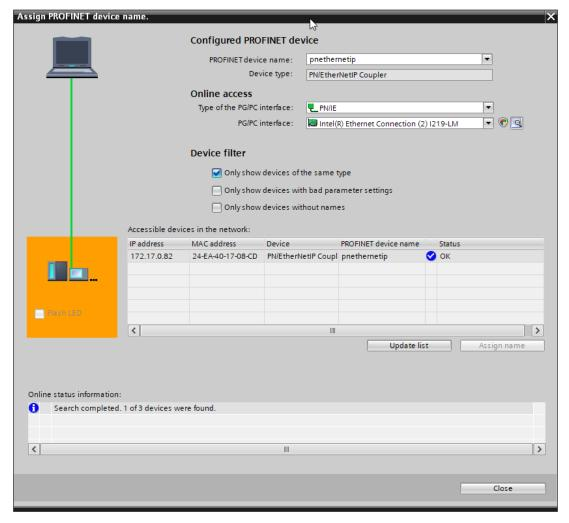
The unique identification of the PN/EtherNetIP coupler is guaranteed here by the MAC address of the device. The PROFINET MAC address can be read on the front of the PN/EtherNetIP Coupler on the left-hand side at X1 ("MAC 1").
