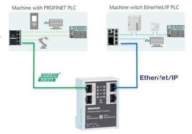
extra configuration software is not necessary. The configuration of the I/O data to be exchanged is carried out in the Siemens engineering tool. An EDS file matching the configuration can then be downloaded from the website by the PN/EtherNetIP Coupler and used to configure the EtherNet/IP PLC.
